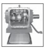
10) Take out plungers and seal sleeves as described above. Drain the oil by taking off the plug (12). After removing the clip ring (33B), lever out the seal retainer (33) with a screwdriver. Open hose adaptor (K11) and remove gear cover (K3). Remove the cooling vane plate (K1) by removing the screws (K4)
